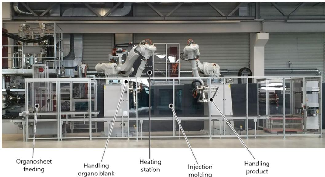
**FIGURE 5** Numerous tests were carried out at the Brose tech center system to find the right process parameters
