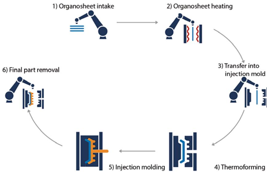
**FIGURE 4** Process steps for manufacturing continuous fiber-reinforced lightweight design components
