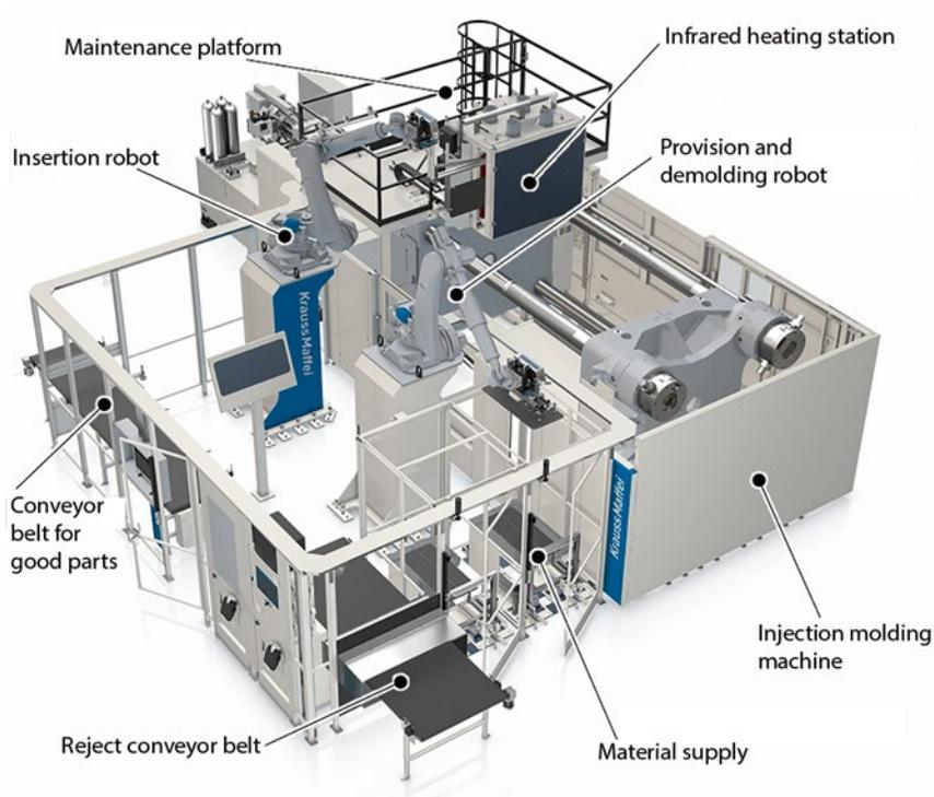
**FIGURE 6** Krauss Maffei manufacturing solution for manufacturing door modules in organosheet design (© Krauss Maffei)
