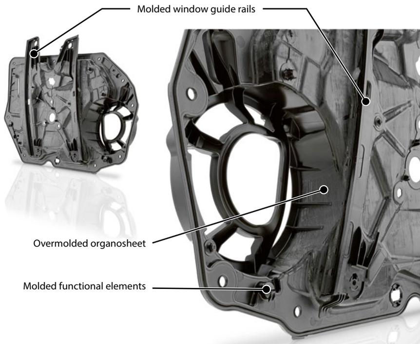
FIGURE 3 The developed organosheet door module carrier (© Brose | Krauss Maffei)
