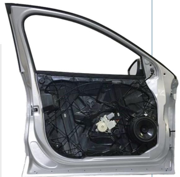
**FIGURE 7** The new Brose door module carrier concept (© Brose)
