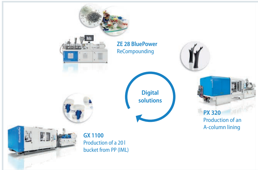
Fig. 1. A bucket becomes an A-pillar: at K2019, KraussMaffei is demonstrating a closed material and manufacturing cycle composed of extrusion and injection molding technology in combination with digital solutions (© KraussMaffei)
