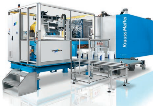
Fig. 2. The speed option of the new GX 1100 ensures high speeds during injection and fast mold movements
